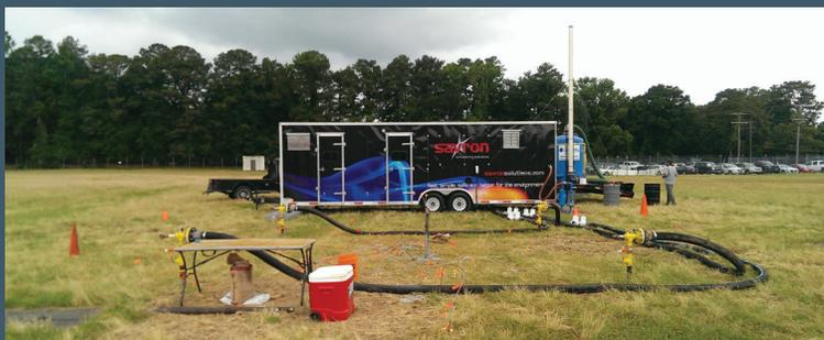
**IMAGE 1:** PDE test area showing the ignition/air injection well, associated thermocouple network, and the STAR control trailer.
