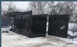
**IMAGE 1:** 10 m<sup>3</sup> pilot Hottpad system designed to evaluate treatment efficiency, processing rate, and emissions treatment requirements
