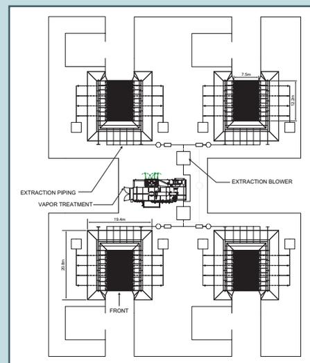
**IMAGE 3:** Treatment plant consisting of four (4) Savron HP-200 base units (200 m<sup>3</sup> volume each) can treat approximately 135 tonnes of soil per day.
