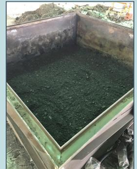
**IMAGE 2:** Petroleum hydrocarbon-impacted silts loaded into Pilot Hottpad™ #1.
