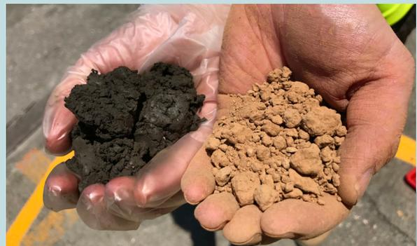
**IMAGE 3:** Silts before and after STARx treatment.
