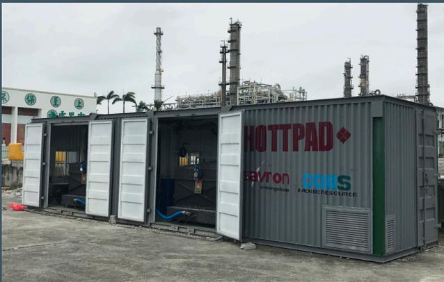
**IMAGE 1:** Dual Hottpad™ pilot system each with a capacity to treat approximately 1.2 m<sup>3</sup> of soil.
