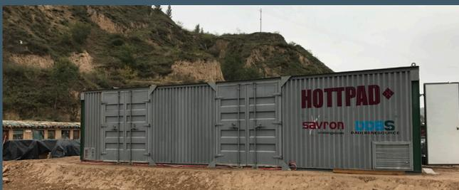
**IMAGE 2:** Dual Hottpad™ pilot system installed within a shipping container for rapid mobilization
