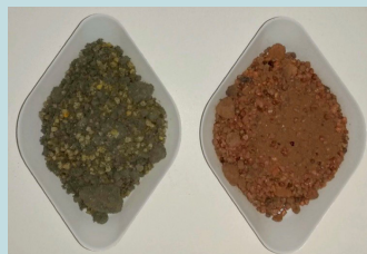
IMAGE 2: Untreated tailings sample (left) and smoldered tailings sample after STARx treatment (right)
