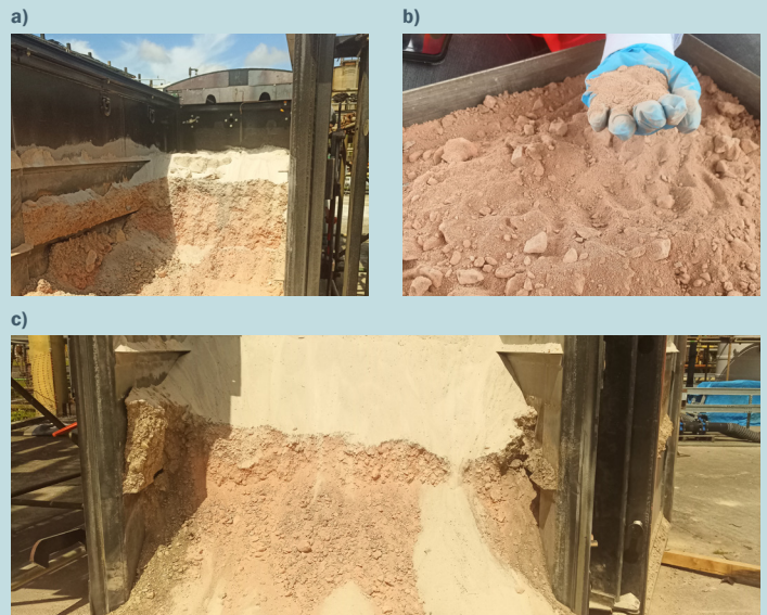
IMAGE 3: Site soils following STARx treatment using different surrogate fuels to support the combustion process: a) GAC; b) eucalyptus bark; and c) coconut husks.
