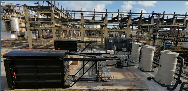
IMAGE 2: Dual Hottpad™ pilot system showing the two 10m 3 treatment vessels and the vapor extraction and treatment system (Granular Activated Carbon [GAC]).
