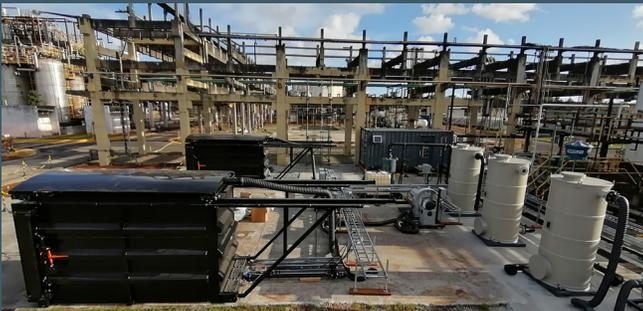
**IMAGE 2:** Dual Hottpad™ pilot system showing the two 10m<sup>3</sup> treatment vessels and the vapor extraction and treatment system (Granular Activated Carbon [GAC]).
