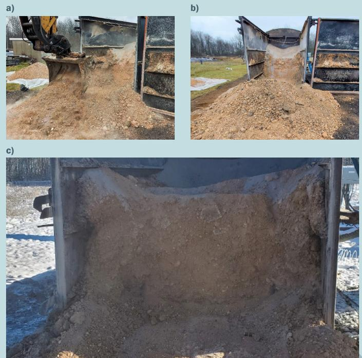
**IMAGE 3:** Site soils following STARx treatment from: a) Test 1 front of Hottpad, b) Test 1 rear of Hottpad; and c) Test 2.
