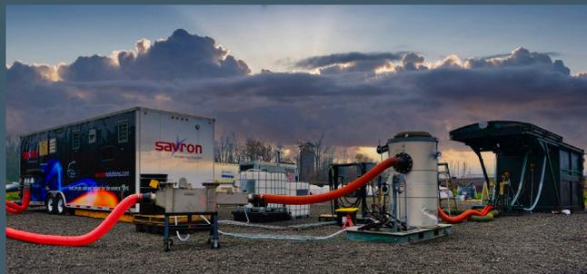
**IMAGE 2:** Pilot system setup, including (from left to right): Hottpad vessel, injection / extraction auxiliary equipment, control trailer, generators / fuel cubes, and emissions extraction and treatment system (granular activated carbon [GAC]).
