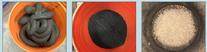
**IMAGE 2:** Combined primary and waste activated sludge sample (left), mixture of sludge and sand before STARx treatment (centre), and remaining sand after STARx treatment (right)
