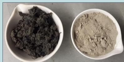
**IMAGE 4:** Pulp and paper residue prior to STARx treatment (left) and ash remaining after STARx treatment (right)
