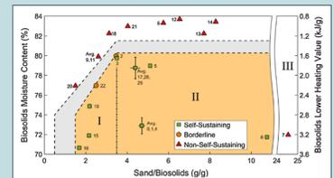
**IMAGE 3:** Parameter space illustrating sludge ('biosolids') moisture content, lower heating value, and sand/biosolids mass ratio combinations that facilitate self-sustained smoldering (Rashwan et al., 2016)
