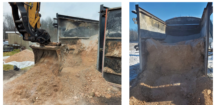
IMAGES 2a and 2b: Site soils following STARx treatment during unloading from Test 1 and Test 2.
