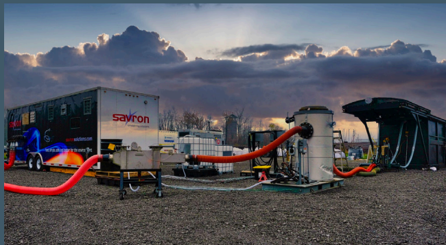
IMAGE 1: Pilot system setup, including (from left to right): control trailer, injection/extraction auxiliary equipment, and Hottpad vessel.
